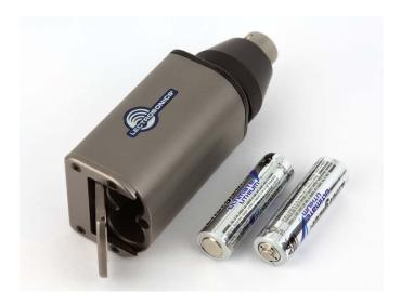
The battery compartment door is hinged to the housing and remains attached to the transmitter when opened. It securely latches in place and applies pressure to the batteries when closed. The two AA batteries are connected in series through a conductive plate on the door.
